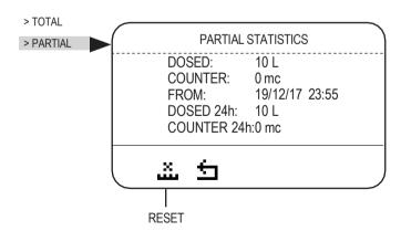
DOSED: total quantity dosed (max 999.999.999 L). COUNTER: water meter counter (cubic meter of water).
